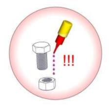
All bolts, nuts, cylinder nuts, etc. (except for Nyloc nuts) must be secured with at least5 drops of Loctite!
