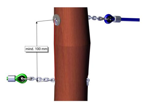
Calculate the drill angles in order not to cross the steel mounting plates !
