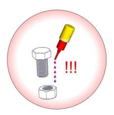
All screws, nuts (except stop nuts) and sleeves must be and sleeves must be secured with Loctite!
