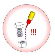
glue all screws, nuts and sleeves with loctite. (not less than 5 drops!) (except for lock nut)
