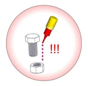
Glue all screws, nuts and sleeves with loctite. (not less than 5 drops !) (except for lock nuts)
