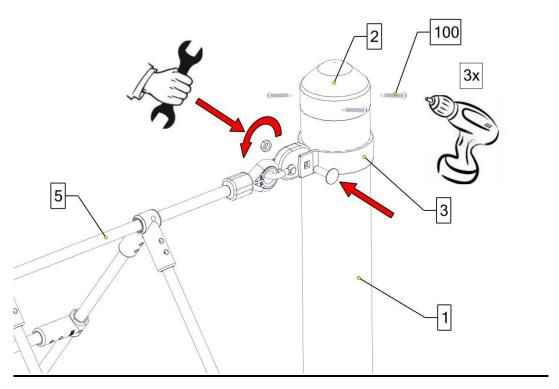
Fixed anchor/plug fastening for M12-15-30 /110
