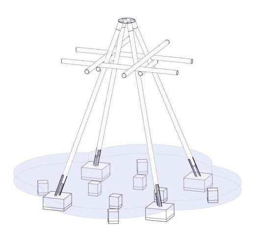
Place the wooden frame in the prepared foundation recesses and align it vertically.
