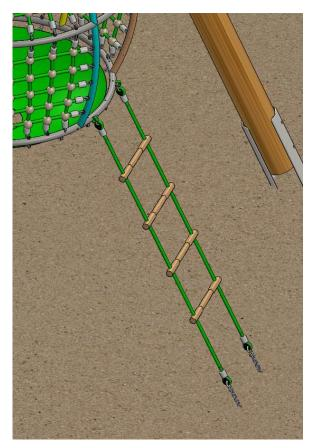
The meshes are marked with A,B,C,D and are assigned to the corresponding olive. (see page 15). The assembly is carried out using the preassembled shackles and one plastic bushing each, which are installed in the metal bushings of the olive / Mini-M nest.
