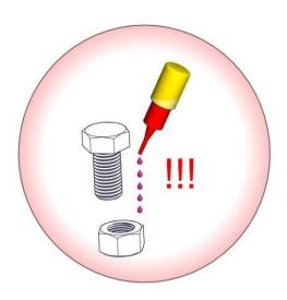
glue all screws, nuts and sleeves with loctite.
